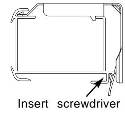
Gently pry the screwdriver to release the bracket from the headrail. Take care not to damage the painted finish of the headrail.
