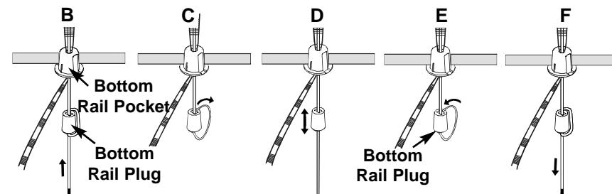
Follow the same procedures for adjusting the middle moving rail on a top down/bottom up shade.
