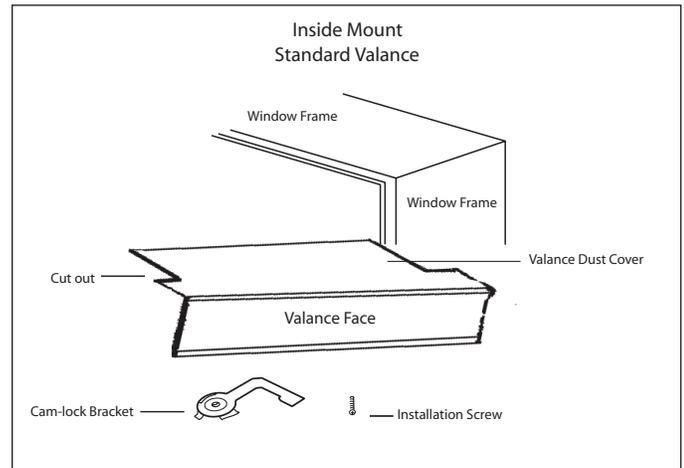
**\*CAUTION -cam-lock brackets should not be more than 4" from either side. Begin by mounting the left and right brackets and center any remaining brackets between them. Valance brackets may need to be adjusted for minimum depth applications.**
