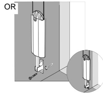
2) Fully extend tensioning device. Lock into extended position by rotating the post 45 degrees.
