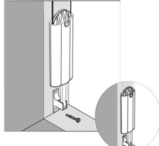
Use wall anchor to hold mounting screw in place, if needed.
