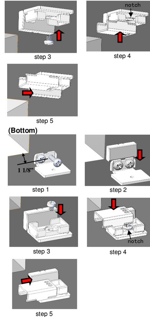
Note: See below. Align L bracket 1/4" away from the edge to outside screw hole of the L bracket.
