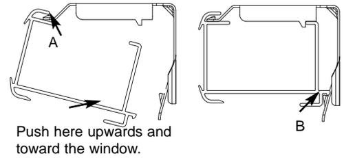
Be sure the motor wire is not pinched by the bracket.
