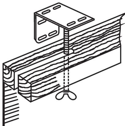
3. Mark the position of brackets at the window with a pencil ensuring all brackets are aligned.
