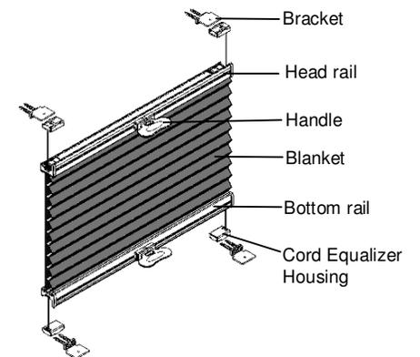
Note: See below. Align L bracket 1/4" away from the edge to outside screw hole of the L bracket.
